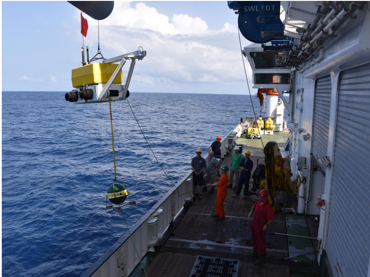
One of the remote seismometers deployed by University of Southampton scientists in the Atlantic Ocean.
